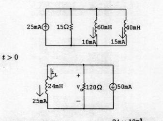
$$i_L(0^-) = i_L(0^+) = 25 \text{ mA}; \qquad \tau = \frac{24 \times 10^{-5}}{120} = 0.2 \text{ ms}; \qquad \frac{1}{\tau} = 5000$$
